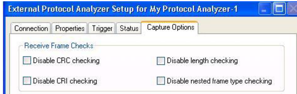
Figure 64 Receive frame checks in capture
